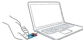
03 Connect stopped logger directly to USB port
